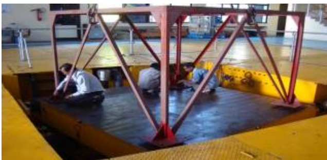
FITTING THE 3D-STEEL FRAME ON THE SHAKE TABLE USING BOLTS
