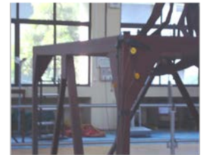
At the specified locations on the scaled model accelerometers are mounted as shown in the figures. During testing the output of accelerometers are recorded as acceleration response. Three accelerometers are fixed in the three mutually perpendicular directions.
